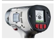
The LITHIUM SERIES II Tool incorporates TorcSense™Technology which directly measures torque providing more repeatable results. Now available in a 5000 ft-lbs configuration expanding the operational capability of this tool. With all new features such as the sliding directional switch, snug function, user access levels, advanced bolting, and more further extends the versatility of the tool.
