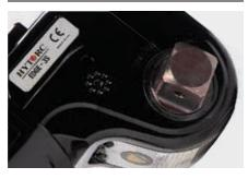
For quick and simple directional changes, the EDGE S splined square drive can be removed and installed on the opposite side with no tools. Hex Drives and other Direct Drives are also available with the EDGE S tool SAFETY HANDLE
